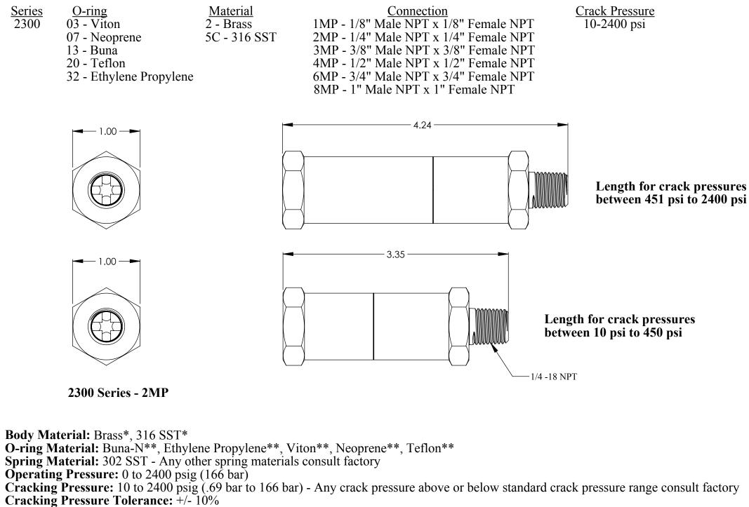
**Temperature Range:** -70 °F to +400 °F (-56 °C to +204 °C) - Based on o-ring and body material **Connection Sizes:** (1/8" MNPT x 1/8" FNPT to 1" MNPT x 1" FNPT)\*\*\*
